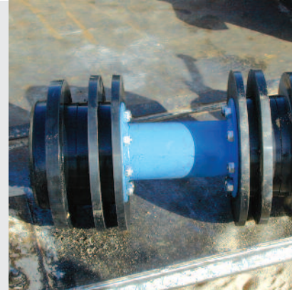
Pigging tool prior to cleaning run
