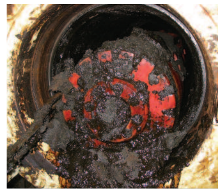
Wax removed from a 14" line with a dual module cleaning tool
