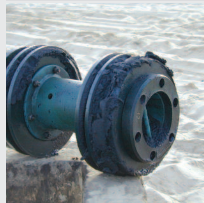
Pigging tool after cleaning run
